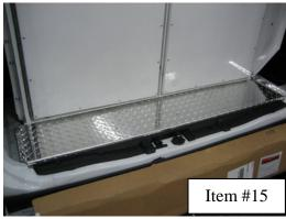
Place trim panels as shown above Pre-drill through trim panel (only) with 3/16". Pre-drill the vehicle w/ 1/8" hole and attach panels using #10 x 1" sheet metal screws
